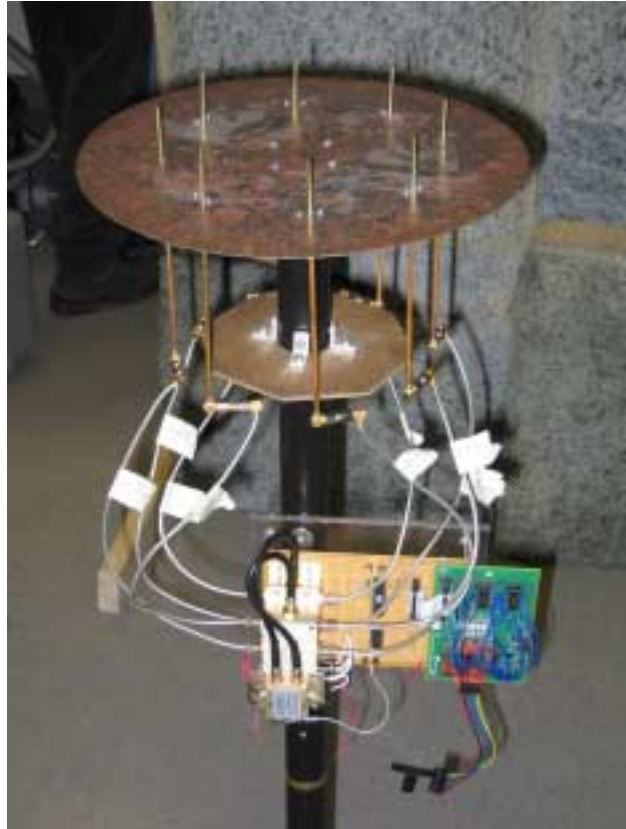
Figure 1.1 MPRG Eight Element Circular Antenna Array
