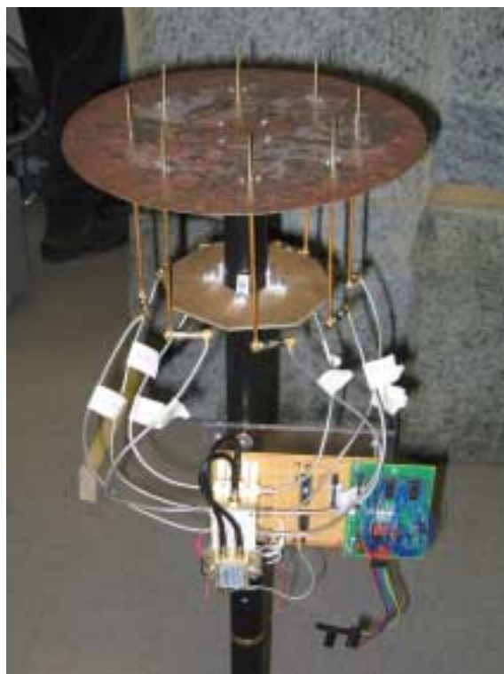
Figure 5.3 MPRG Eight Element Circular Antenna Array
