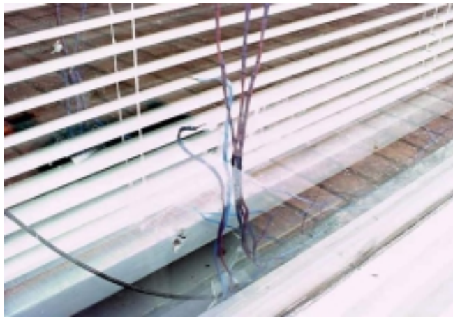
Figure 4.10 Thermocouples are attached to or suspended from the glass surface The thermocouple locations are shown in Figure 4.11, 4.12 and given in Table 4.1.
