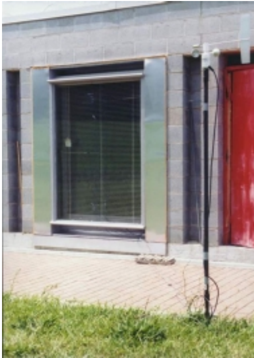
Figure 4.13 Anemometer for wind speed and direction measurement
