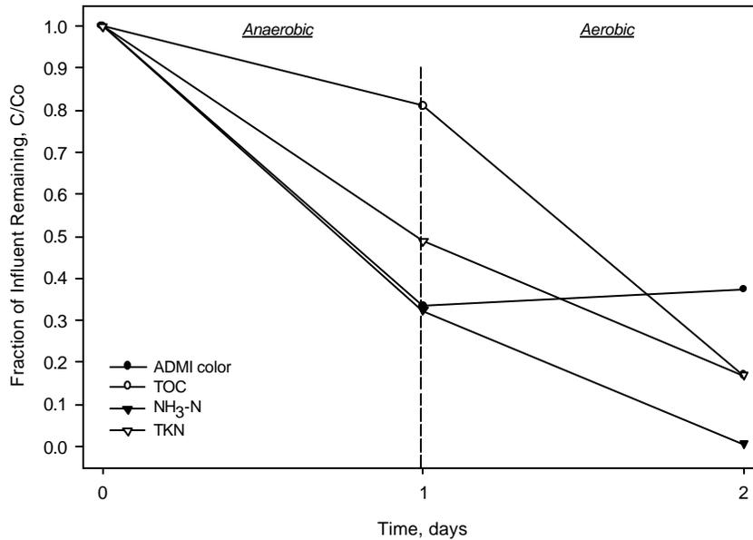
**Figure 23:** Phase IV: Test #1: Biodegradation of POTW influent using ANA/AER sequential step-treatment batch reactors with laboratory acclimated anaerobic sludge and POTW activated sludge.
