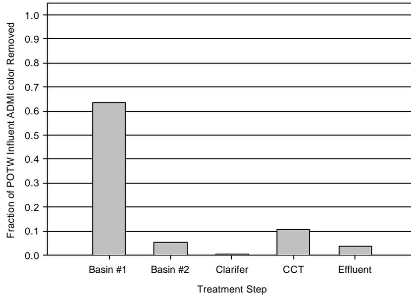
**Figure 25:** Fraction of POTW influent ADMI color removed from wastewater following various treatment steps. Data represents an average of the values recorded during the months of February 2001 and April 2001.
