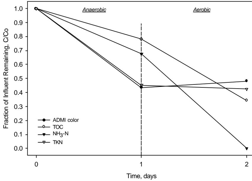
**Figure 22:** Phase IV: Test #1: Biodegradation of POTW influent using ANA/AER sequential step-treatment batch reactors with laboratory acclimated sludges.
