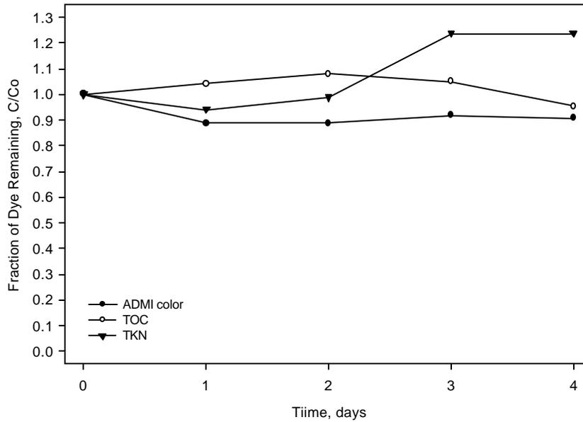
**Figure 19:** Phase III: Test #3: Aerobic reduction of Cypress Green dye ADM color, TOC, and TKN using batch reactors with an initial dye concentration of 2ml/L.
