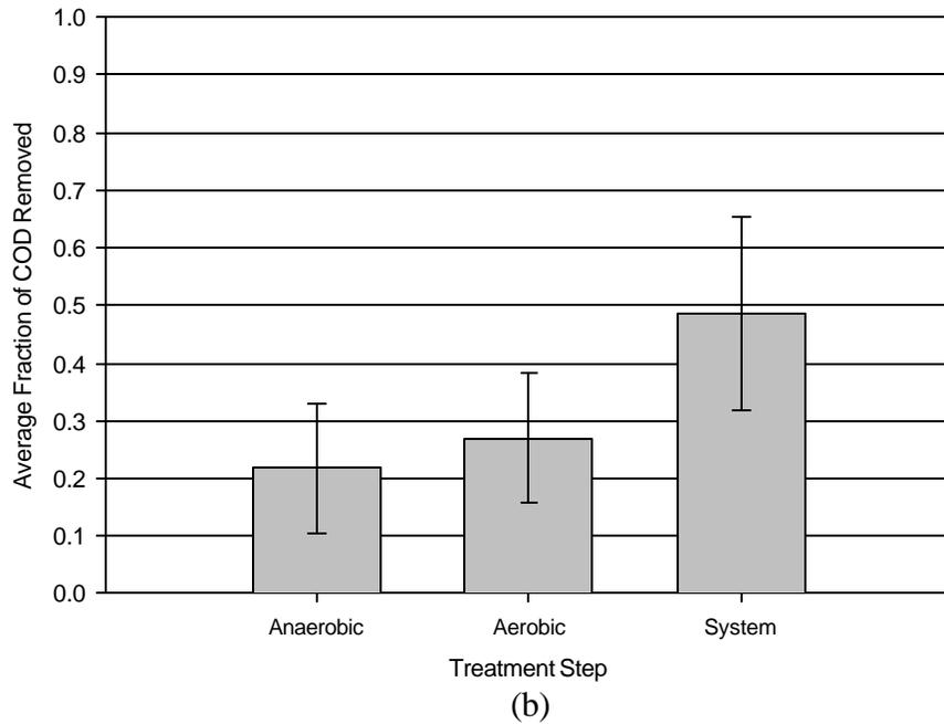
**Figure 11:** *Phase II: Test #1:* (a) Cypress Green dye COD removal following each step of ANA/AER sequential step-treatment. (b) Average fraction of COD removed during each step of ANA/AER sequential step-treatment. (Standard deviation,  $n=2$ )
