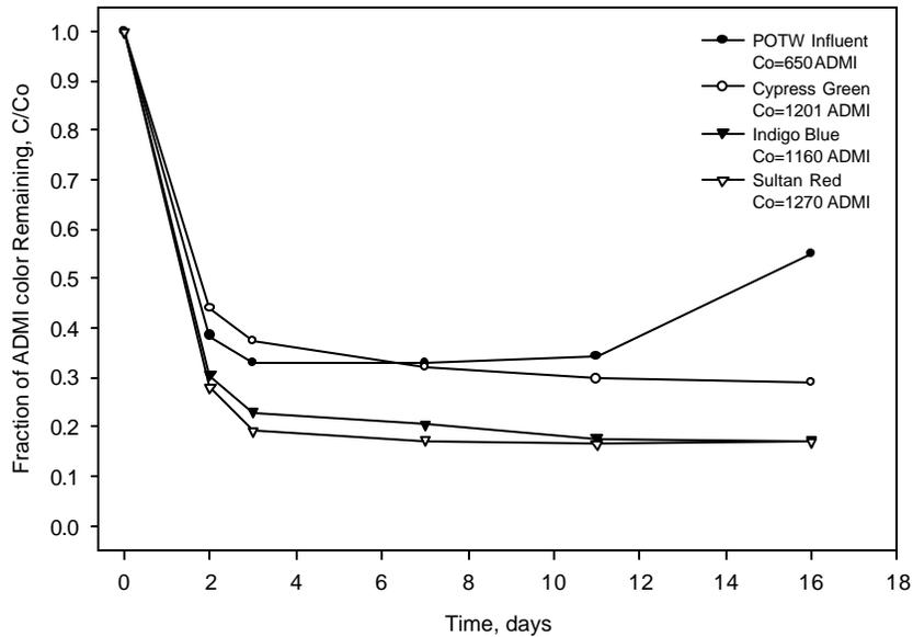
**Figure 5:** Phase I: Test #2: Anaerobic biodegradation of Cypress Green, Indigo Blue, Sultan Red, and POTW influent ADM1 color using Pepper's Ferry digester sludge.
