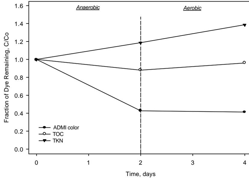
**Figure 20:** Phase III: Test #3: Reduction of Cypress Green dye ADMI color, TOC, and TKN using ANA/AER sequential step-treatment batch reactors with an initial dye concentration of 2ml/L.
