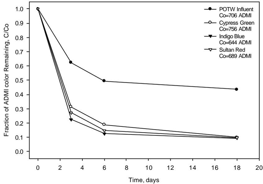
**Figure 6:** *Phase I: Test #3:* Aerobic biodegradation of Cypress Green, Indigo Blue, Sultan Red, and POTW influent ADMI color using POTW activated sludge.
