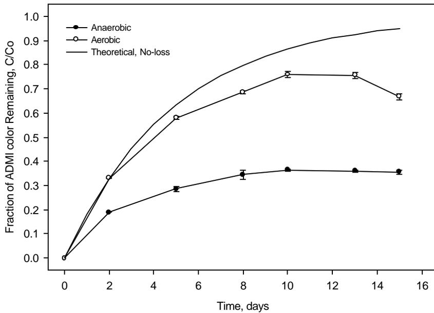
**Figure 15:** *Phase III: Test #1:* Anaerobic versus aerobic Cypress Green dye ADM1 color loss. (Standard deviation,  $n=2$ )
