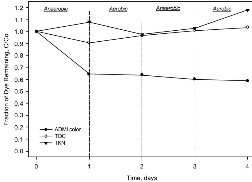
**Figure 21:** *Phase III: Test #3:* Reduction of Cypress Green dye ADMi color, TOC, and TKN using ANA/AER/ANA/AER sequential step-treatment batch reactors with an initial dye concentration of 2ml/L.
