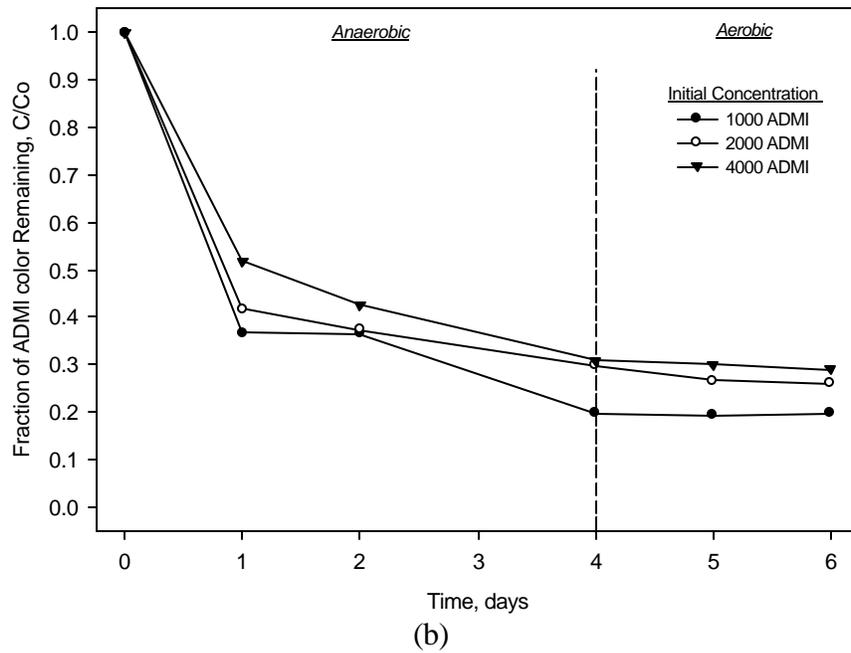
**Figure 13:** Phase II: Test #2: (a) Cypress Green dye ADMI color loss using anaerobic TSS concentration of 8000 mg/l, followed by aerobic TSS concentration of 2000 mg/L. (b) Cypress Green dye ADMI color loss using anaerobic TSS concentration of 4000 mg/l, followed by aerobic TSS concentration of 1000 mg/L.
