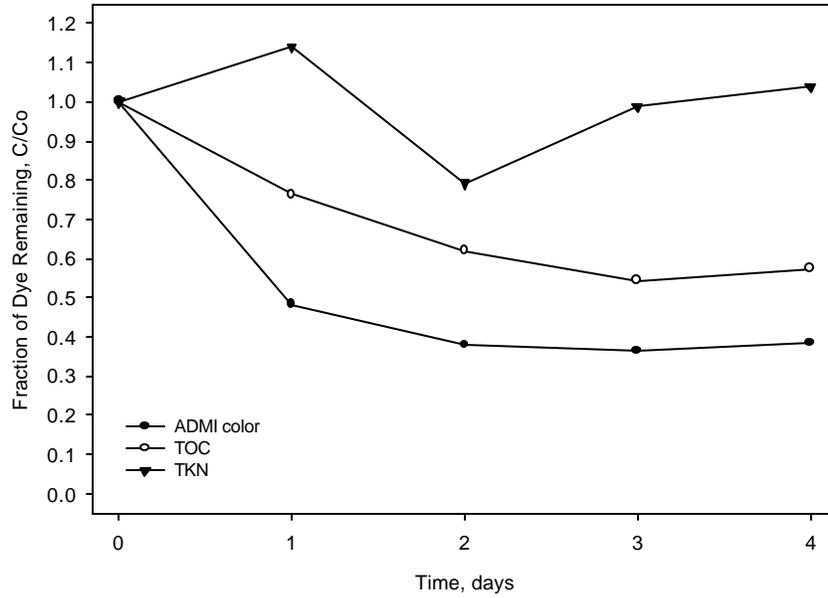
**Figure 18:** Phase III: Test #3: Anaerobic reduction of Cypress Green dye ADM color, TOC, and TKN using batch reactors with an initial dye concentration of 2ml/L.
