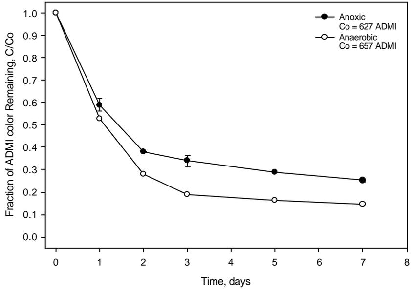
**Figure 7:** *Phase I: Test #4:* Anoxic versus anaerobic biodegradation of Indigo Blue ADMI color using Pepper's Ferry digester sludge. (Standard deviation, n=2)
