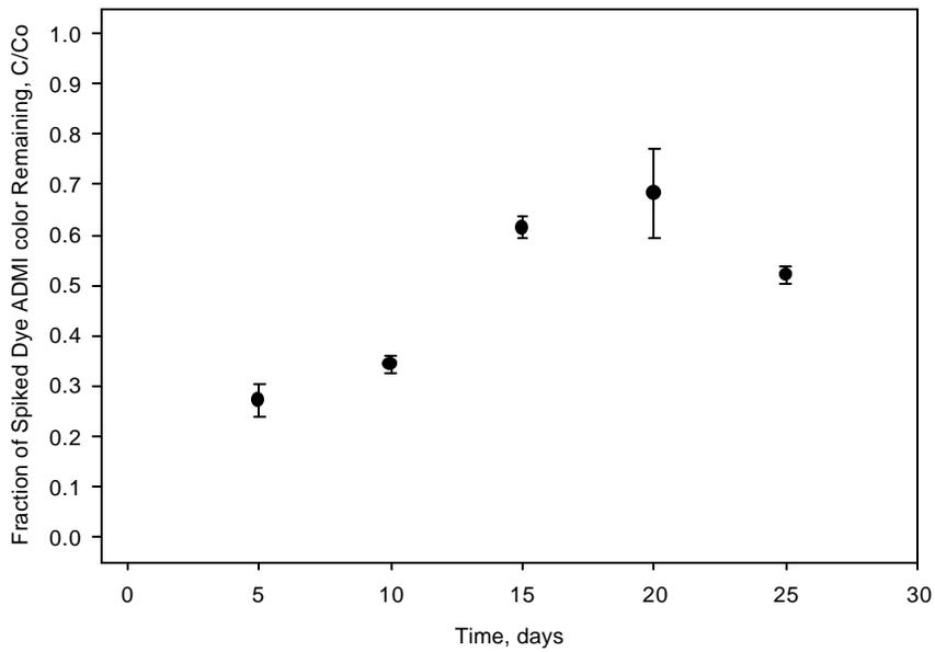
**Figure 8:** *Phase I: Test #5:* Anaerobic ADMI color removal of Sultan Red/Cypress Green/Indigo Blue mixed-dye solution using Pepper's Ferry digester sludge. Reactors were spiked with dye on days 0, 5, 10, 15, and 20. (Standard deviation, n=3)
