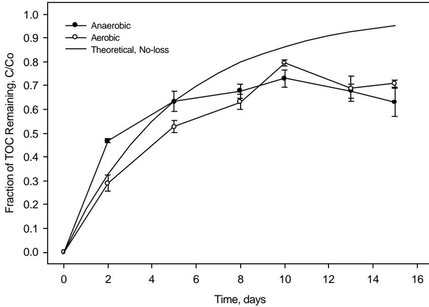
**Figure 16:** *Phase III: Test #1:* Anaerobic versus aerobic Cypress Green dye TOC removal. (Standard deviation, n=2)
