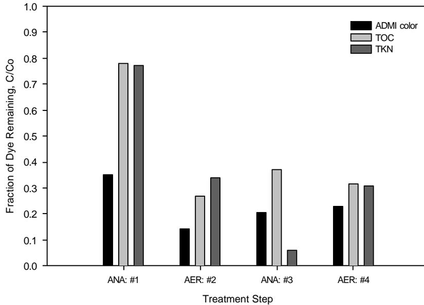
**Figure 17:** *Phase III: Test #2: ANA/AER/ANA/AER sequential step-treatment of Cypress Green dye. The reported ADMi color, TOC, and TKN reductions were taken on day 15 of treatment system operation.*
