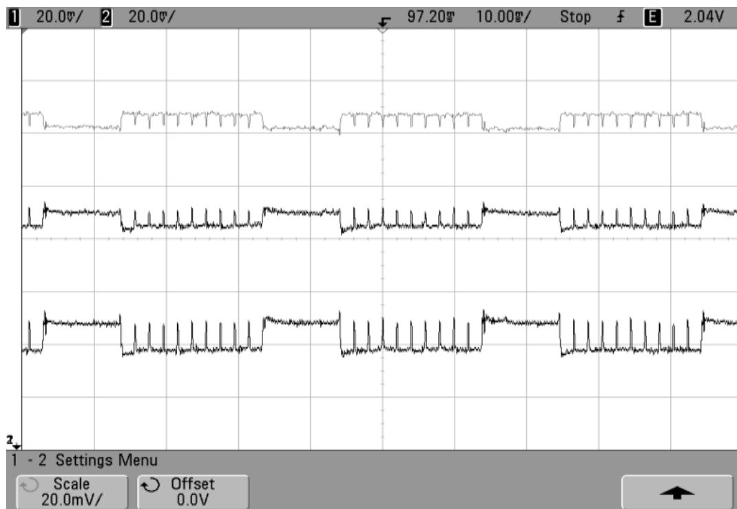
Figure 11. Power Trace of Point Multiplication with ARM+DSP Version
