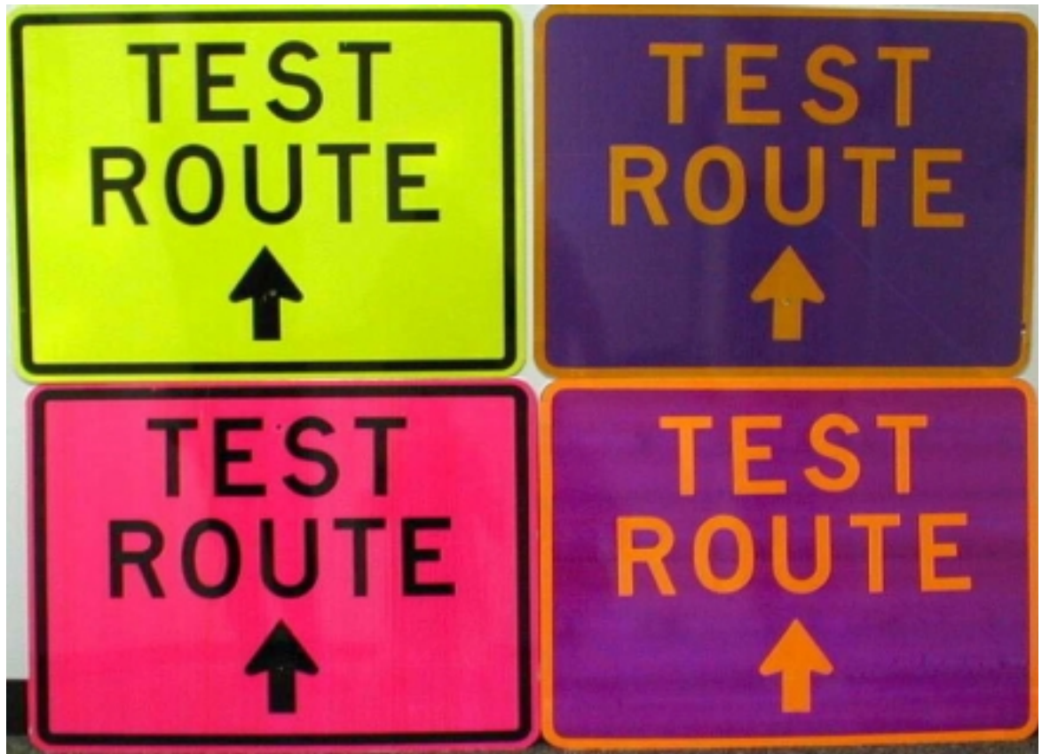
Figure 2. The experimental test signs (clockwise from top left: black on fluorescent yellow-green, non-fluorescent yellow on non-fluorescent purple, fluorescent yellow on fluorescent purple, and black on fluorescent coral).
