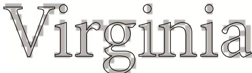
The word "Virginia" is shown in a smooth, serif font. The letters are semi-transparent, revealing a light gray grid underneath. This illustrates how the smooth curves of the font do not perfectly align with the discrete pixels of the raster grid.
