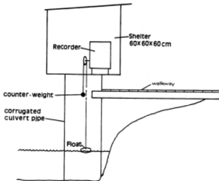
**Figure 3.3.** Typical recording stage-gage installation (Mostaghimi et al., 1989)
